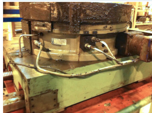
Rotary table before refurbishment
